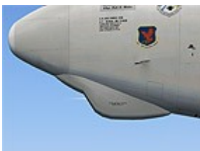
Nose warning antenna
