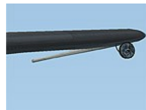
Retractable landing lights (2)
