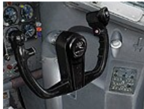
Control wheels and columns (2)
