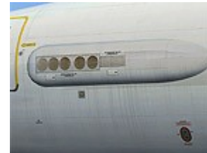
Electronic Support Measure
